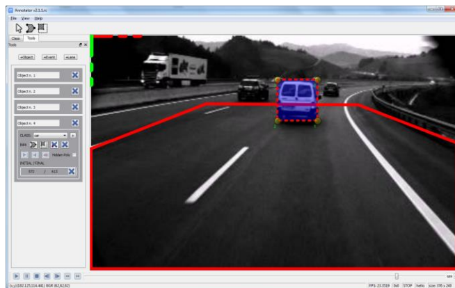
Figure 7 - Vehicle samples annotation for Collision Avoidance Systems.
