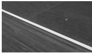
Fig. 3 High shutter speed (1/500). Electronic gain enabled. Blur-free Ball
