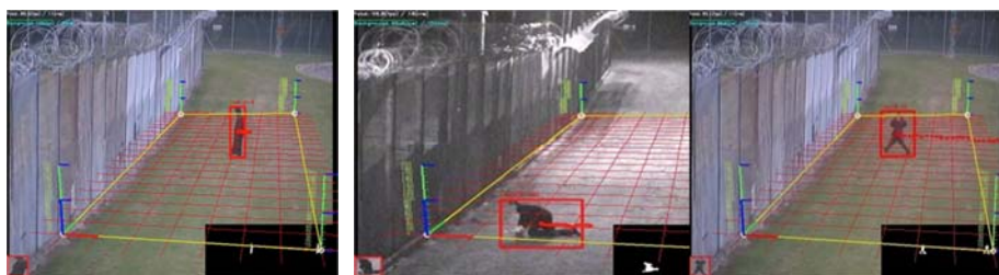
Figure 8: Blob detection can trigger launching “Person Walking”, “Person Crawling” or “Person Running” events in surveillance applications.
