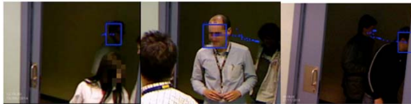
Figure 6: Detection of People and estimation of their trajectory to determine “Person Enters” and “Person Exits” events.
