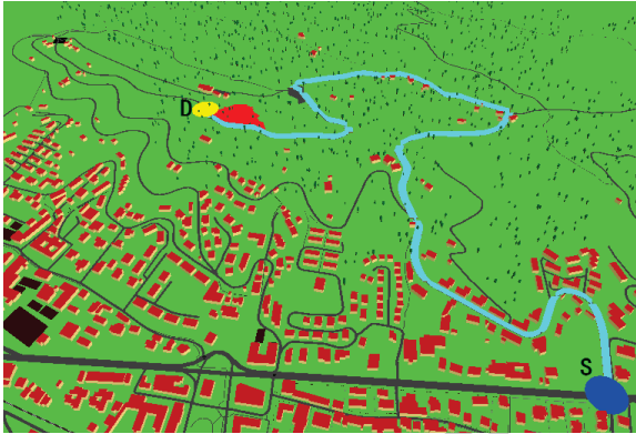
Figure 6: The calculated paths (speed=30, 50 km/h) from source S (in blue) to destination D (in yellow) through the environment with one fire-affected area (in red)
