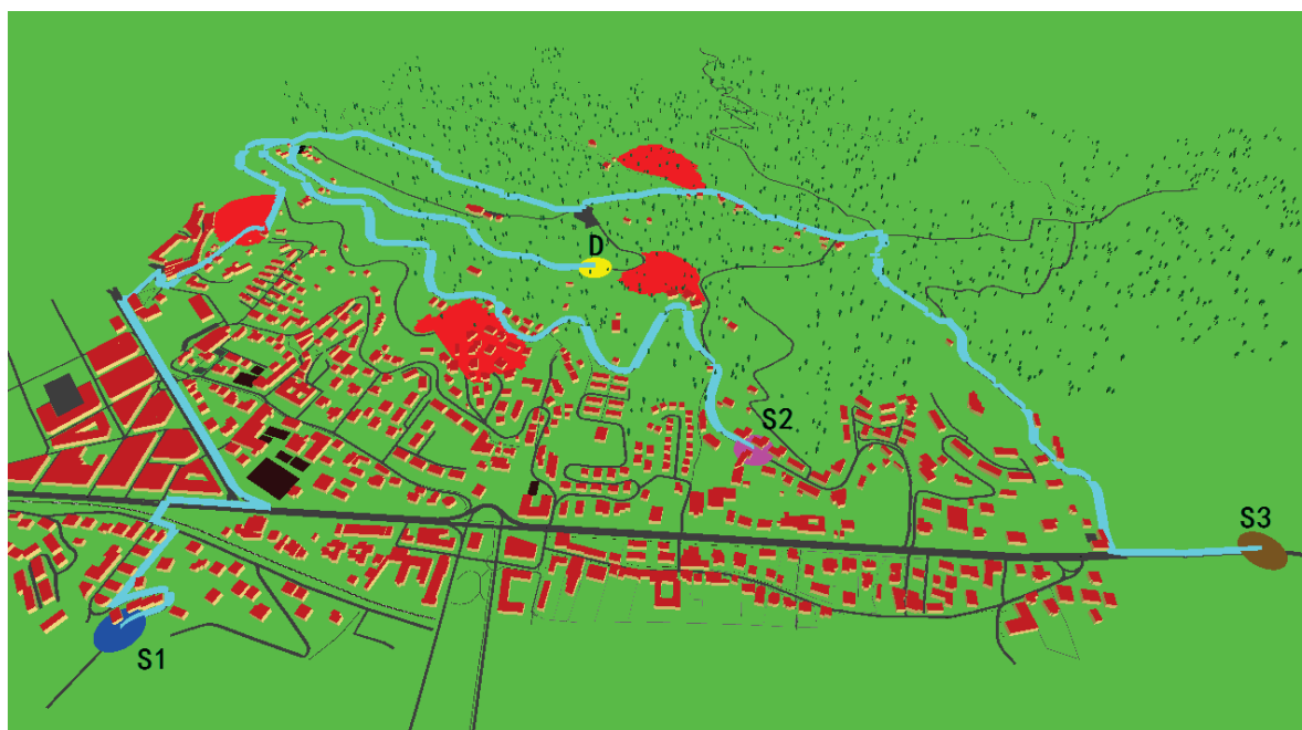
Figure 7: The calculated paths for three vehicles among multiple fire-affected areas (Vehicle 1 from source S1 (in blue) to destination D (in yellow); Vehicle 2 from source S2 (in purple) to destination D (in yellow); Vehicle 3 from source S3 (in brown) to destination D (in yellow))
