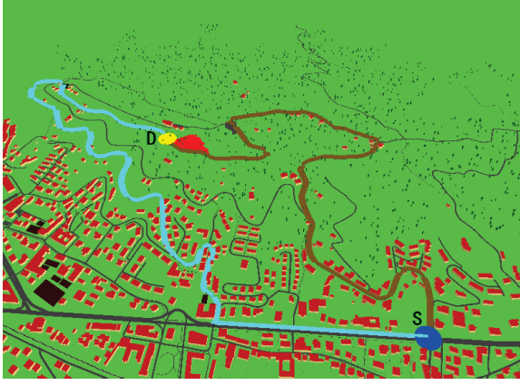
Figure 5: The calculated paths (speed=20 km/h) from source S (in blue) to destination D (in yellow) through the environment with one fire-affected area (in red)
