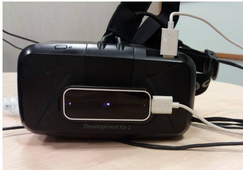
Figure 2: Leap Motion Controller attached to Oculus Rift DK2.
