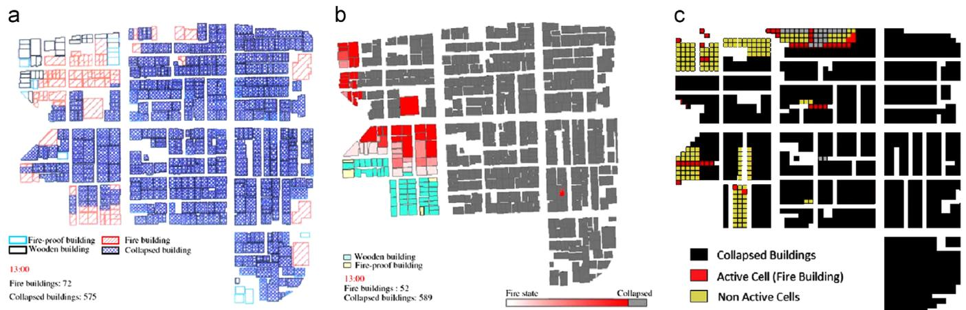
Fig. 16. Validation of urban algorithms. From left to right and top to bottom: (a) real status of the fire after 7 h; (b) Zhao's simulation after 7 h and (c) simulation output with our algorithms.
