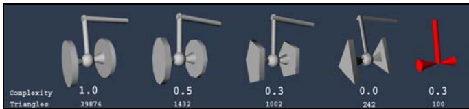
Figure 5: Valves at different complexities and a Valve-Symbol.
