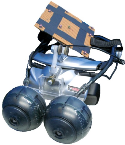
Figure 4: The prototype AR-HMD developed with its front-mounted cameras and a square fiducial marker needed for tracking
