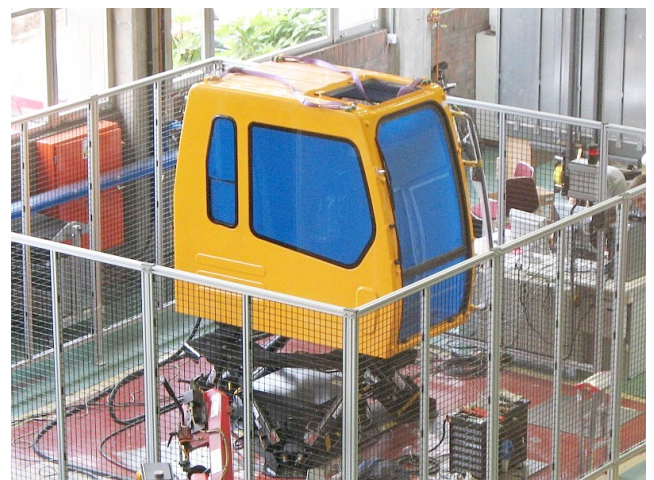
Figure 1: The excavator cabin on the motion platform
