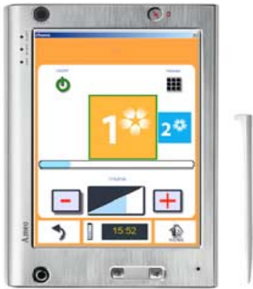
Figure 5. HTC 7500 Advantage controller displaying the Pluggable UI developed for people with cognitive impairments
