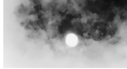
Figure 8: Sky picture looking directly at the sun, taken with an IR camera (spectral range of the camera: 7.5 - 13.5\mu m ).
