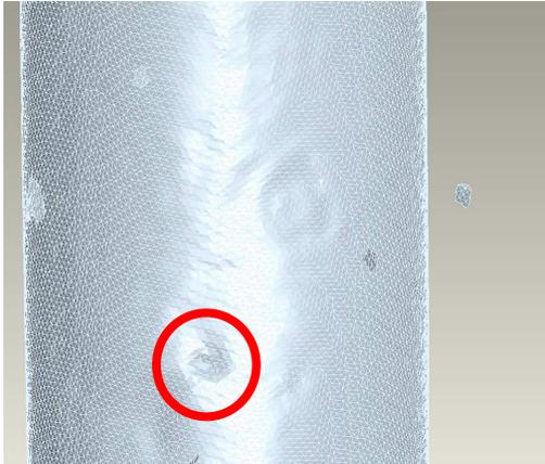
Fig. 3 An example of how a standard 3D scanner cannot detect a hole even if the point cloud density is high enough.
