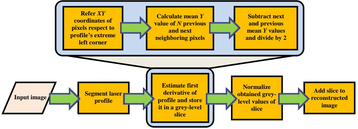
Fig. 6 Tube shape reconstruction diagram.
