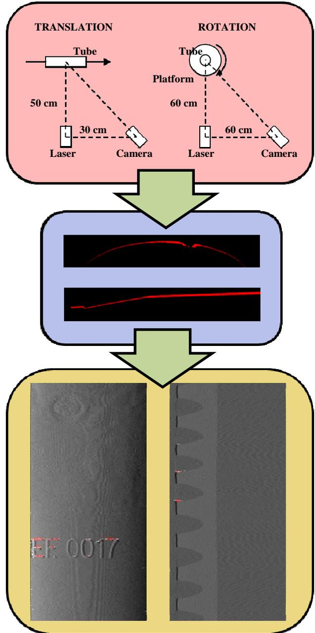
Fig. 5 From top to bottom: the translating and rotating tube system outlines, the observed laser profiles, and the obtained tube shape reconstructions for both systems.
