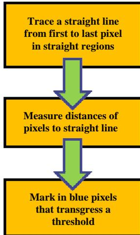
Fig. 8 Deformation detection procedure.
