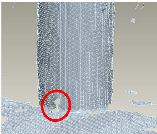
Fig. 4 An example of how a 3D scanner models a burr as a hole.
