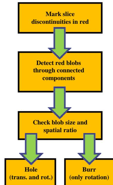
Fig. 7 Hole and burr detection procedure.
