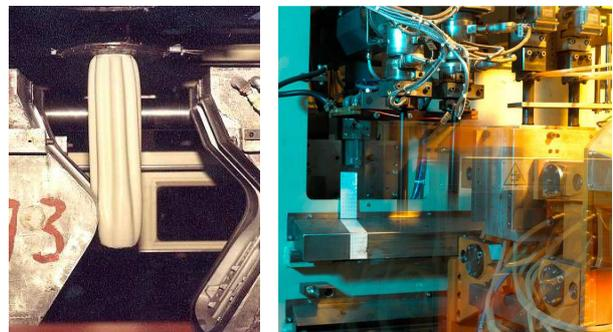
Fig. 1 On the left, a plastic parison falling between the mold's two parts, and on the right, the REINER blowing machine for tubes used as outer covers of car dampers [17].
