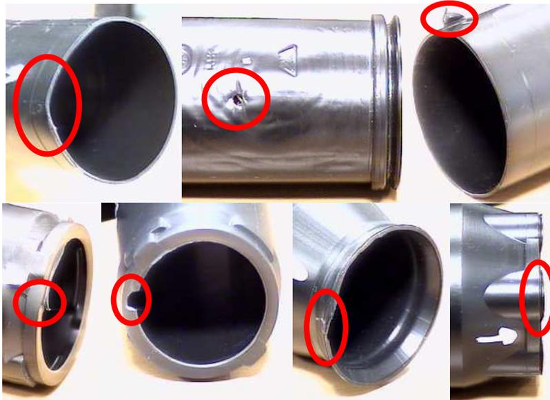
Fig. 2 From left to right and top to bottom: a deformed tube, a hole, a burr and diverse defective cuts.
