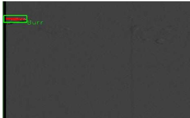
Fig. 10 Burr automatic detection.
