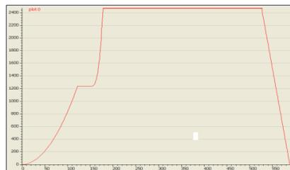
**Fig 11:** Heat (measured in MW) evolution of a wooden unit burning. The unit burnt in approximately 10 minutes. The flash over effect is around 150s.
