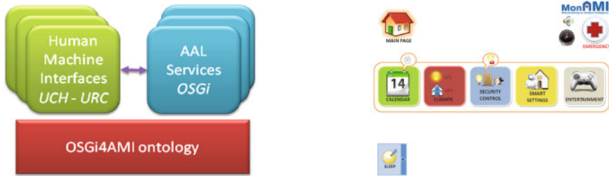
Fig. 3. OSGi4AMI is used both for user interface and for the service definition
