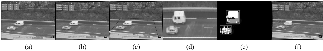
Figure 2: Pre-processing steps: (a) original image; (b) correction of lens distortion; (c) detection of orthogonal directions on the plane; (d) rectified road plane; (e) detected 2D blobs using background segmentation; (f) 3D models after applying the proposed method.
