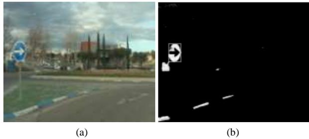
Fig. 12. Image in (b) shows the region detected for image in (a) after color and region analysis.
