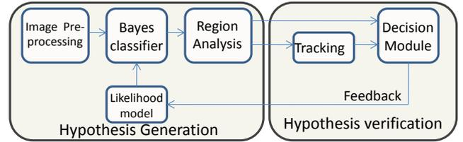
Fig. 1. Block diagram of the proposed TS detection and tracking system.
