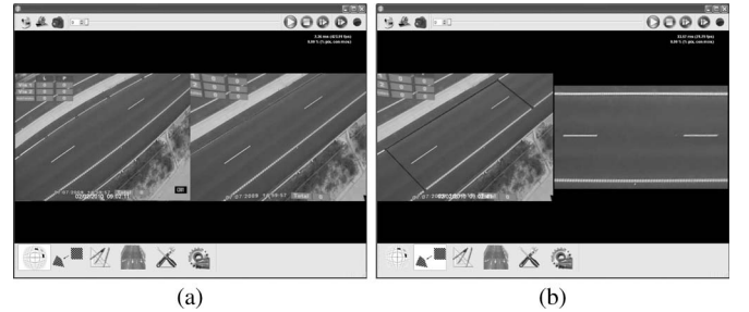
Fig. 11. Results of (a) camera lens distortion correction and (b) perspective correction.
