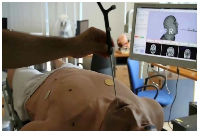
Figure 3: Real-time tracking and 3D representation of the patient for a neurosurgical operation
