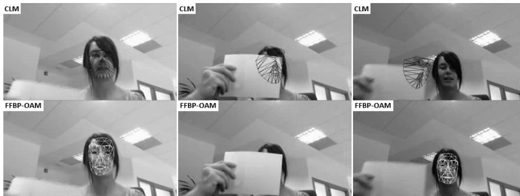
**Figure 3:** Comparison between *CLM* and *FFBP-OAM* on an iPad 2 under a severe occlusion.
