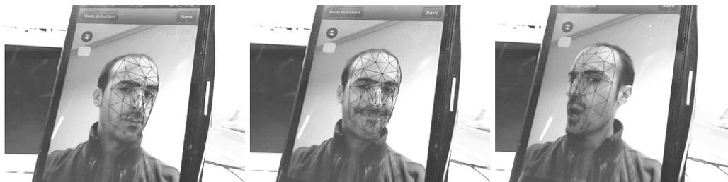
**Figure 4:** The full system running on an iPhone 5 at 24 FPS.
