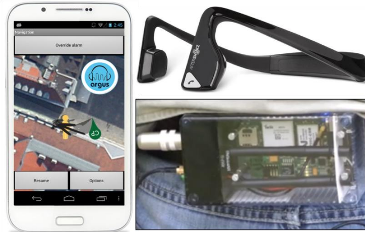
Fig. 2. Pictures of the portable components of the ARGUS prototype: Smartphone running ARGUS App, wireless open headphones and High-Performance Positioning Unit.
