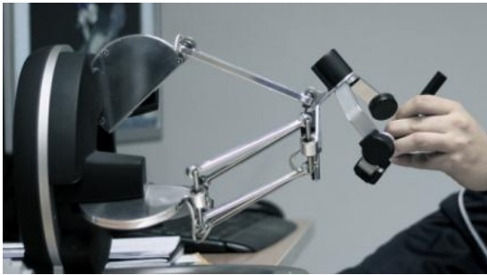
Figure 2. Omega6 haptic device from Force Dimension.
