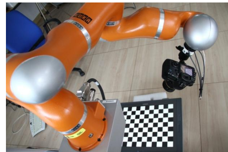
Figure 6. KUKA robot ([17]) in path following mode during the image acquisition process.
