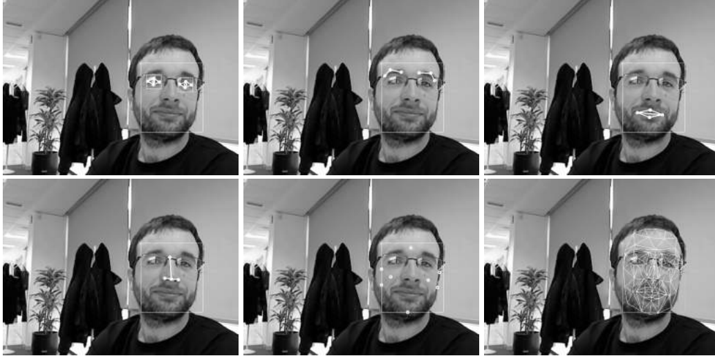
Figure 2: Facial features detection procedure steps. From left to right and top down: (1) eye points detection, (2) eyebrow points detection, (3) mouth points detection, (4) nose points detection, (5) contour points detection and (6) face model fitting on the detected facial features.
