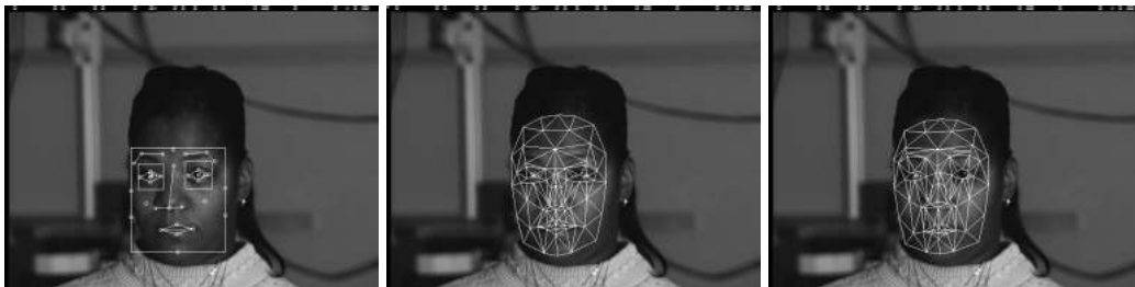
Figure 8: FFBP fitting stages, from left to right: (1) Facial feature detection, (2) POS backprojection (only 3D pose) and (3) LM optimization (3D pose and 15 facial parameters).
