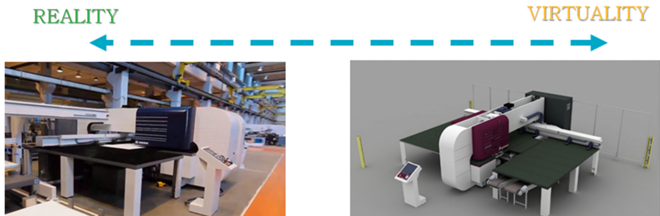
Fig. 3 Digital twins concept: a punching machine in a factory ( left ) and its digital twin ( right )
