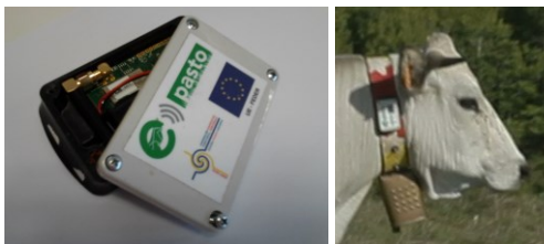
Fig. 3. Developed geolocation devices: general aspect and positioning on the animal's collar.
