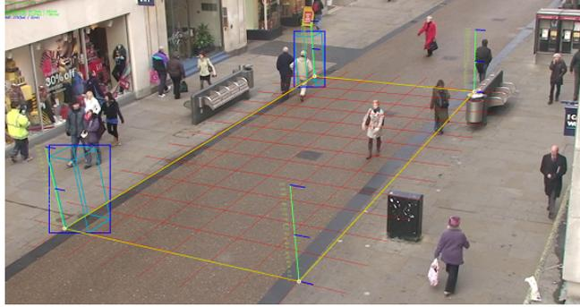
**Fig. 3.** Example use of the GUI for calibrating a typical CCTV scene. The rulers and the projected boxes help to fit the expected sizes of pedestrians.
