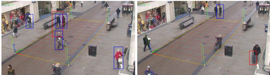
**Fig. 5.** The perspective can be used to filter out detections that do not represent coherent human sizes.
