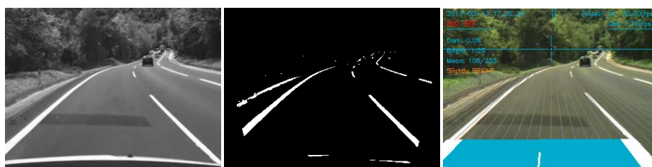
Figure 1: Detection of lane markings and the associated accumulated histogram.
