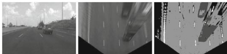
Figure 3: Segmentation process: (left) original image, (center) road-plane image, and (right) four-level segmentation
