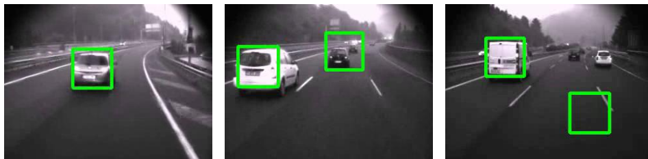
Figure 5: Example results of the detector using SVM and HOG.
